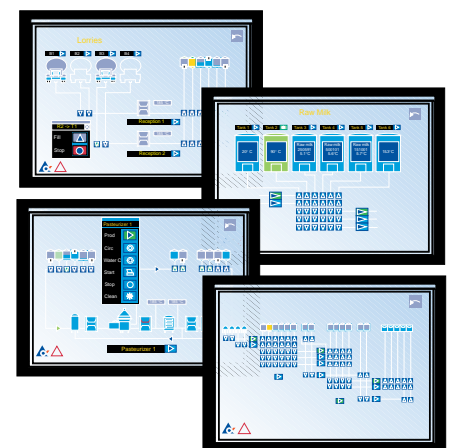
Fig. 6.10.7 Examples of operator information and interaction views on a VDU.
